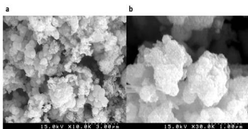
**Figure 3.** SEM image of nanoparticles synthesized with the chemical formula  $Mn_{3-x}Gd_xO_4$  ( $x=0$ (a),  $x=0.08$ (b))
