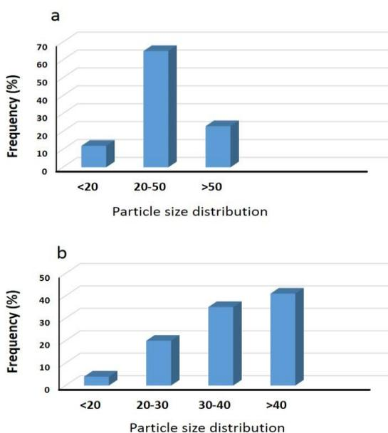
**Figure 4.** Particle size distribution of pure  $Mn_3O_4$  (a) and 8% Gd-doped  $Mn_3O_4$  (b)
