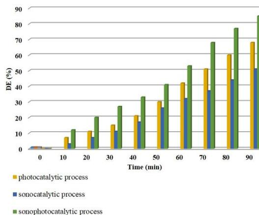
**Figure 5.** Comparison of different processes in the removal of methylene blue dye considering the following conditions: [Dye] = 20 mg/L, [Catalyst] = 1 g/L.
