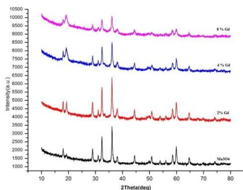
**Figure 1.** P-XRD pattern of manganese oxide doped with gadolinium cation  $Mn_{3-x}Gd_xO_4$  ( $x=0$  to  $x=0.08$ )
