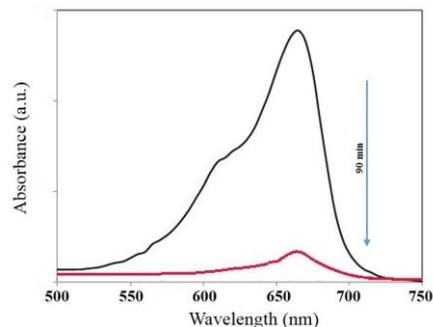
**Figure 6.** Absorption spectrum of color removal in the presence of manganese oxide doped with gadolinium under sonophotocatalysis process.
